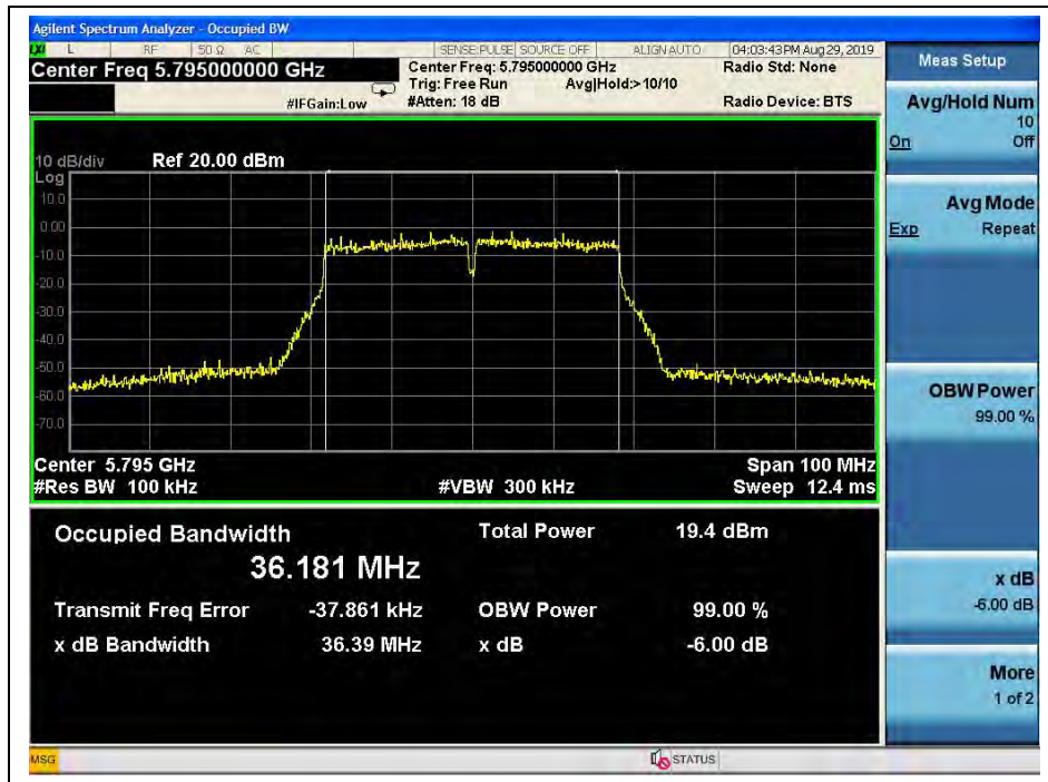
(Channel 159, 5795MHz, 802.11ac (VHT40))
