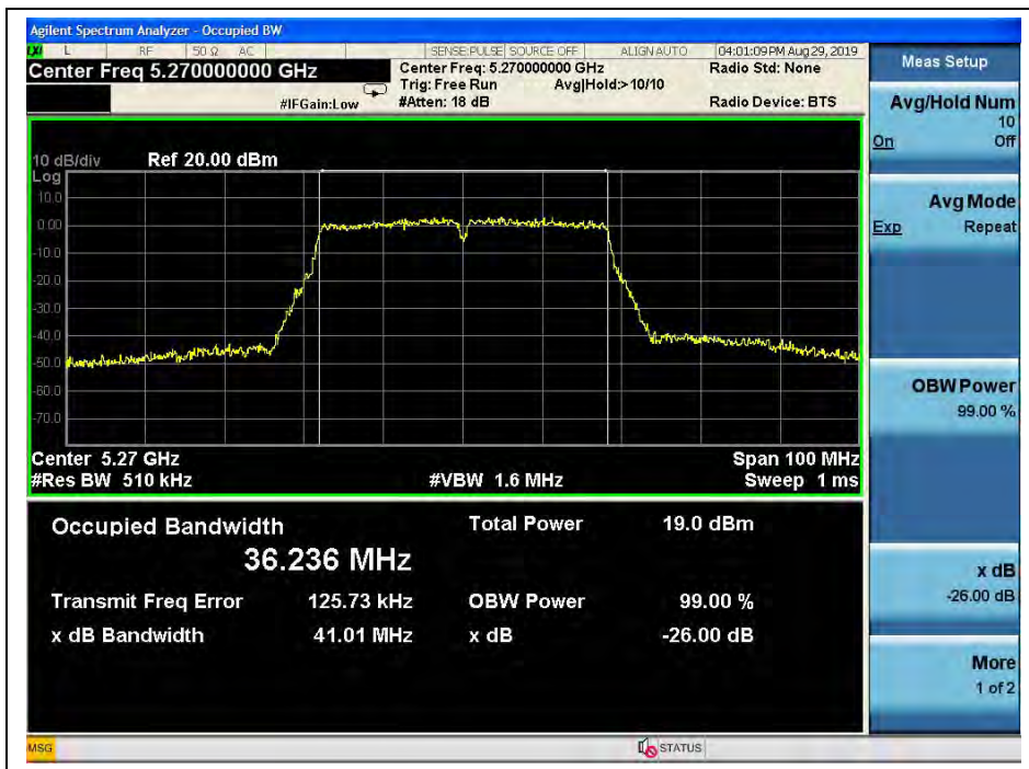
(Channel 54, 5270MHz, 802.11 ac (VHT40))
