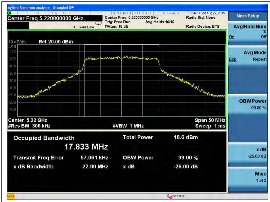
(Channel 44, 5220 MHz, 802.11 ac (VHT20))
