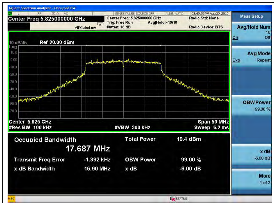
(Channel 165, 5825MHz, 802.11 ac (VHT20))
