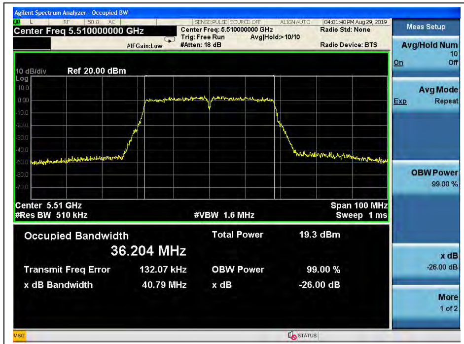
(Channel 102, 5510MHz, 802.11 ac (VHT40))
