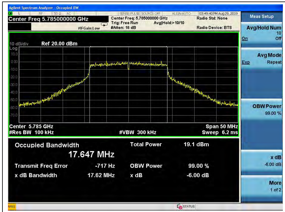
(Channel 157, 5785MHz, 802.11 ac (VHT20))
