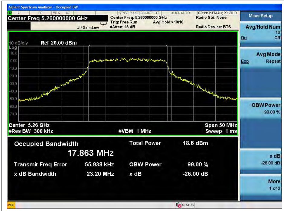
(Channel 52, 5260MHz, 802.11 ac (VHT20))
