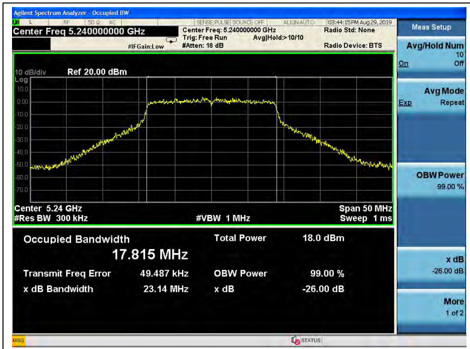
(Channel 48, 5240MHz, 802.11 ac (VHT20))
