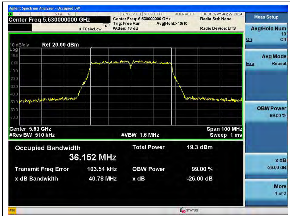
(Channel 126, 5630 MHz, 802.11 ac (VHT40))
