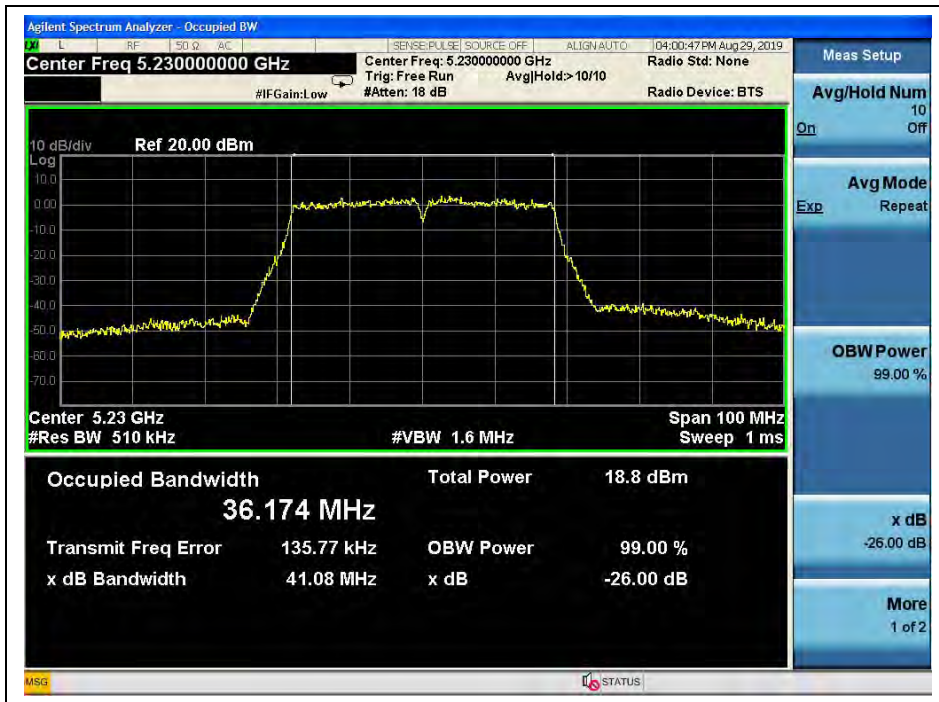
(Channel 46, 5230 MHz, 802.11 ac (VHT40))
