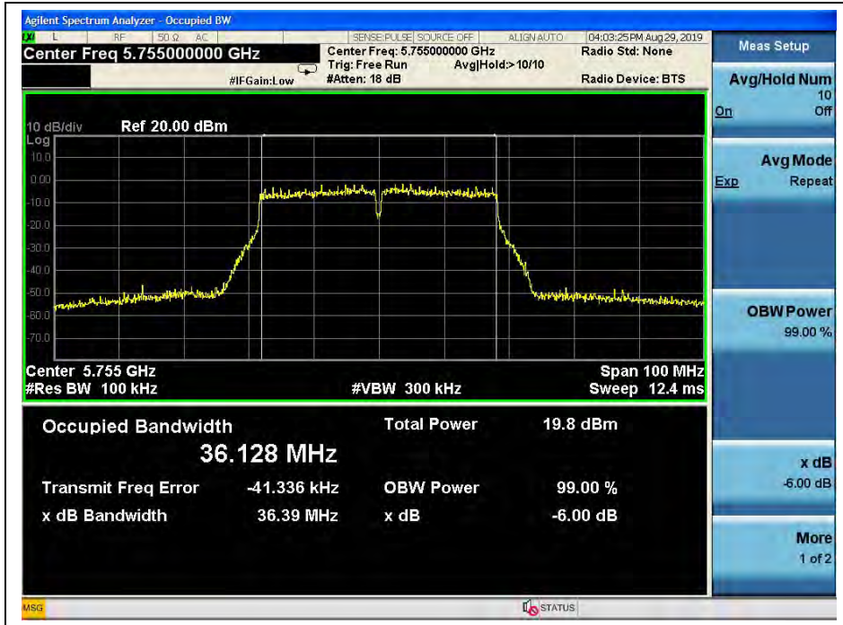
(Channel 151, 5755 MHz, 802.11 ac (VHT40))
