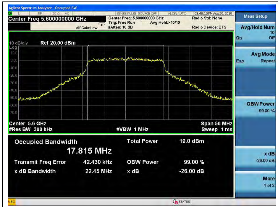
(Channel 120, 5600 MHz, 802.11 ac (VHT20))
