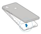
Install the nano-SIM card and the microSDXC card (optional) as shown.
