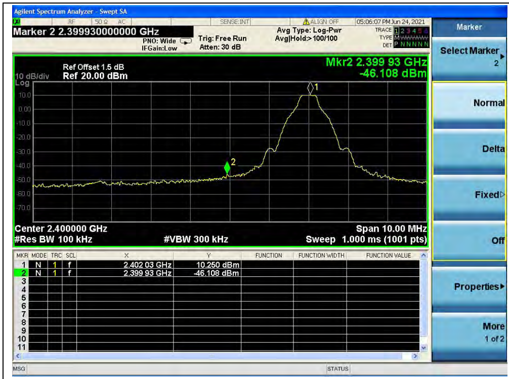
(Band edge, Channel 0, GFSK)
