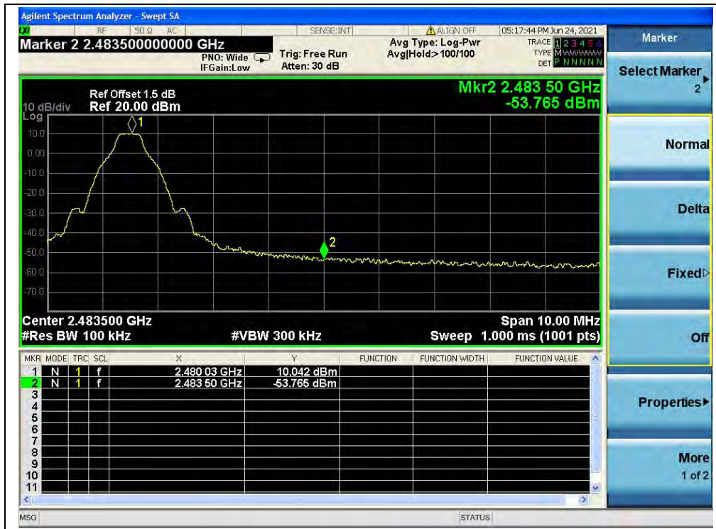
(Band edge, Channel 78, GFSK)
