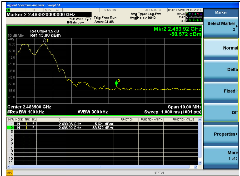
(Band edge with hopping on, Channel 78, GFSK)
