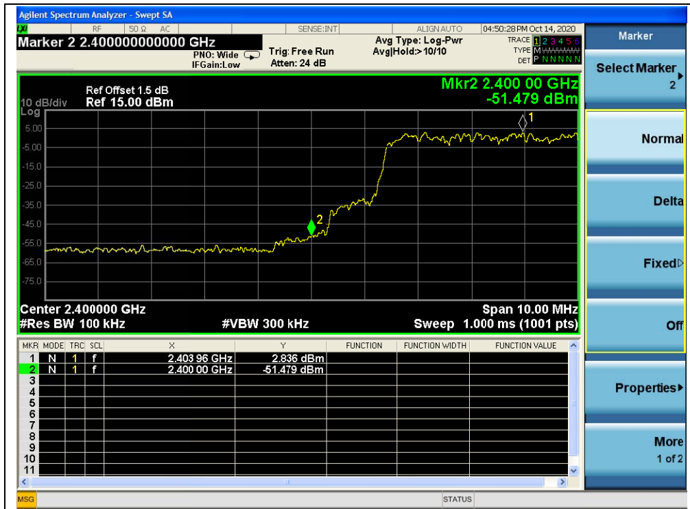
(Band edge with hopping on, Channel 0, 8-DPSK)
