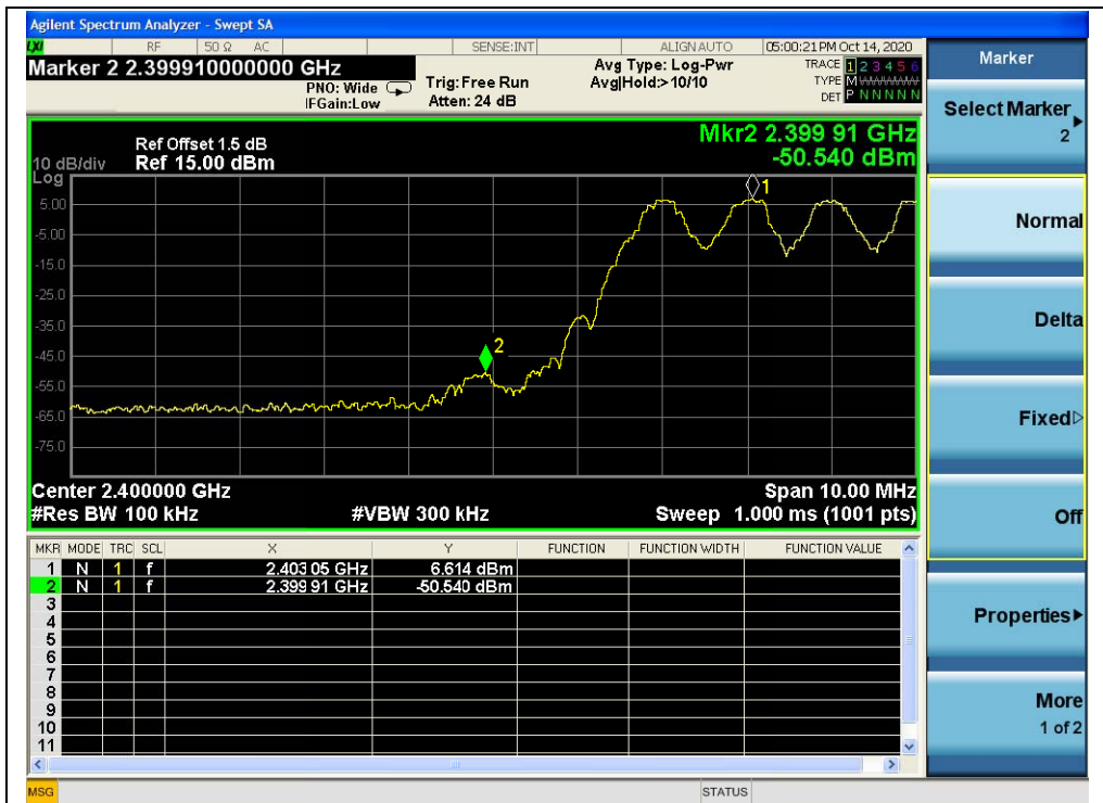
(Band edge with hopping on, Channel 0, GFSK)
