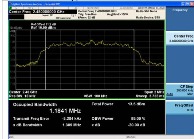
Modulation type: π/4DQPSK 2480MHz
