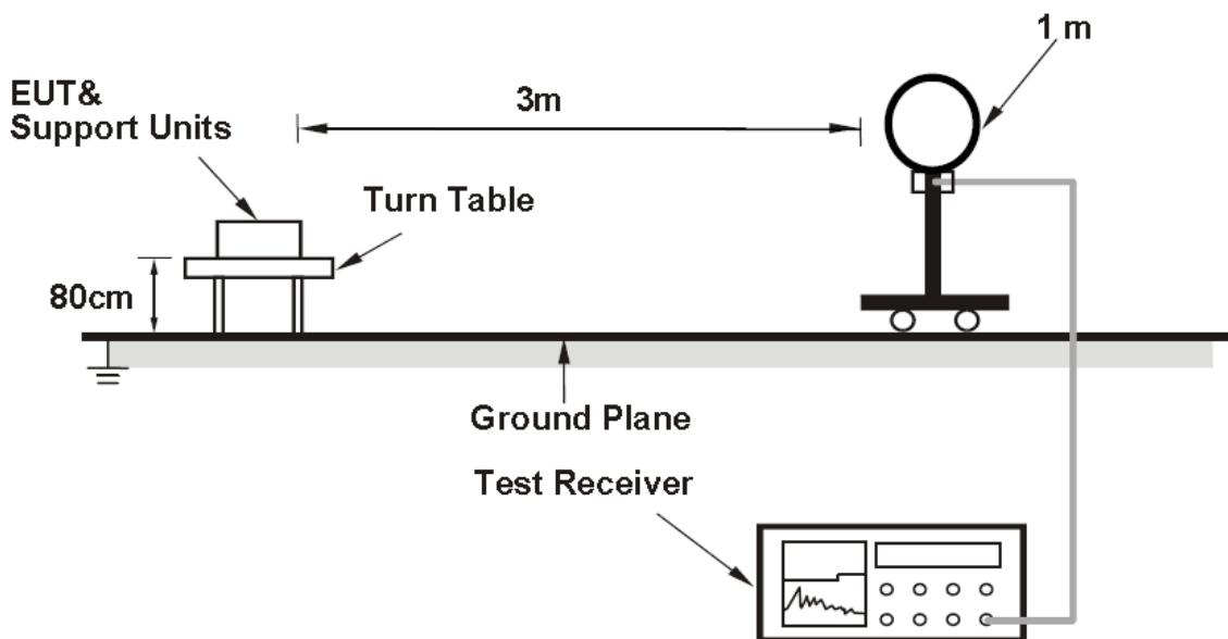
For Radiated emission 30MHz to 1GHz
