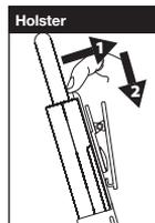
1. Remove Holster by releasing the belt clip latch and sliding the holster downward.
