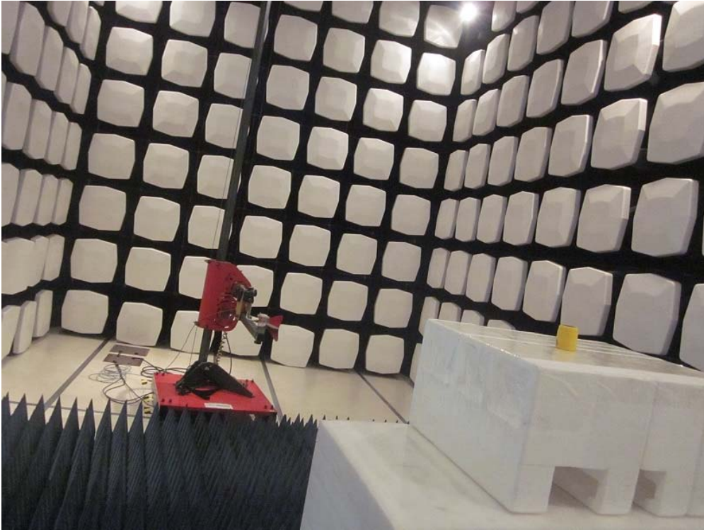
Measurement of Radiated Emission Test Set Up
