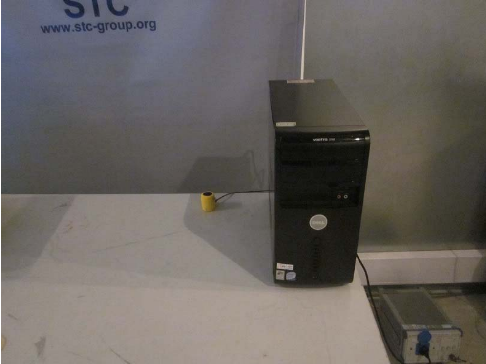
Measurement of Conducted Emission Test Set Up
