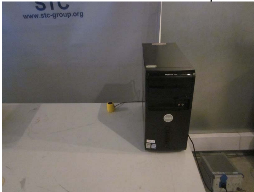
Measurement of Conducted Emission Test Set Up
