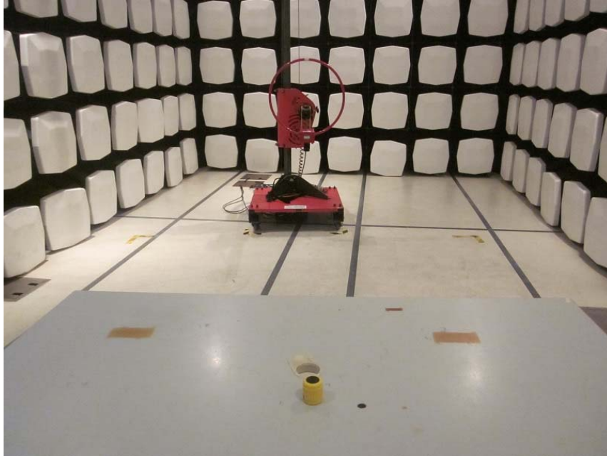
Measurement of Radiated Emission Test Set Up
