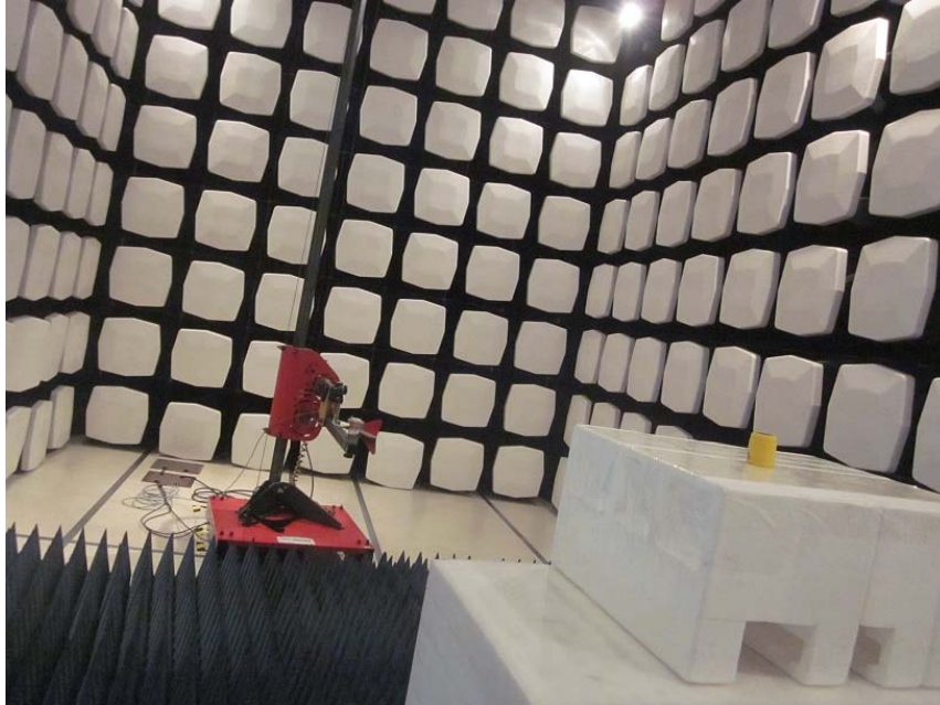
Measurement of Radiated Emission Test Set Up
