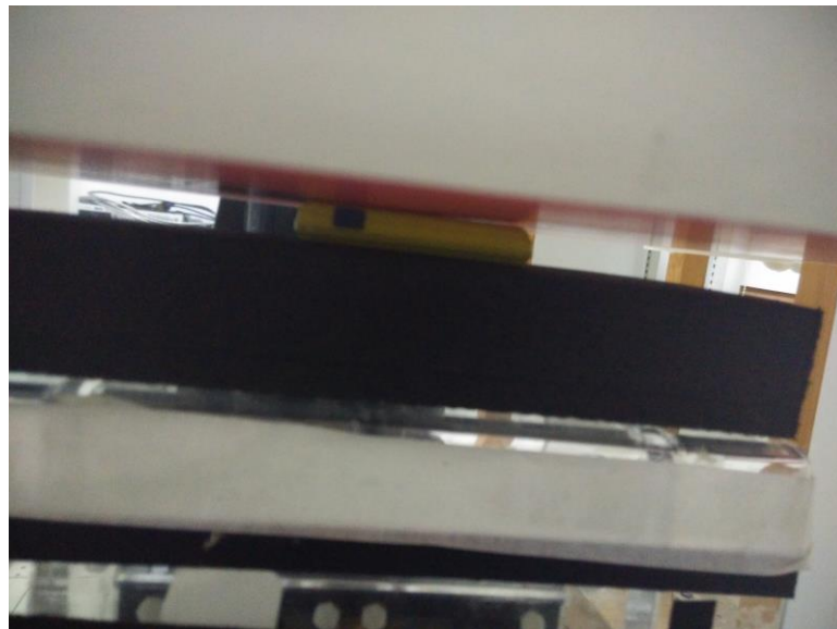
Body-worn Configuration, the back of the EUT towards phantom (The Distance was 0mm)
