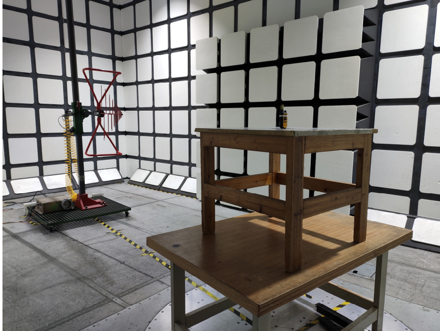
Radiated Emissions View (Below 1 GHz)
