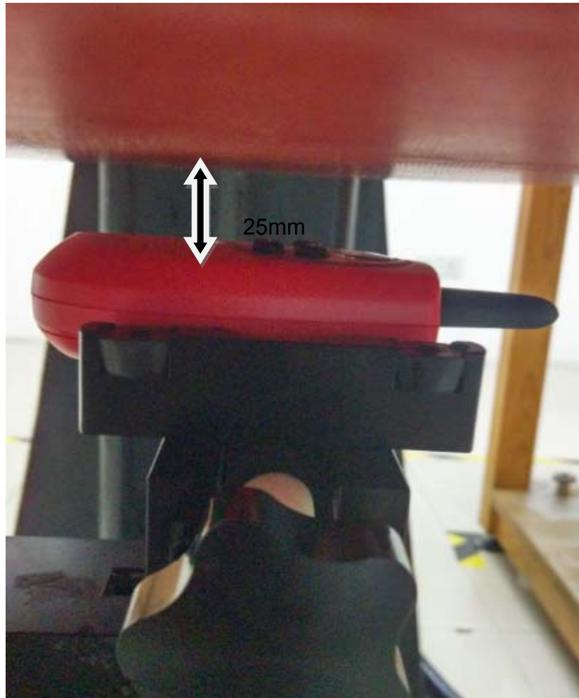
Face-held, the front of the EUT towards phantom (The distance was 25mm)
