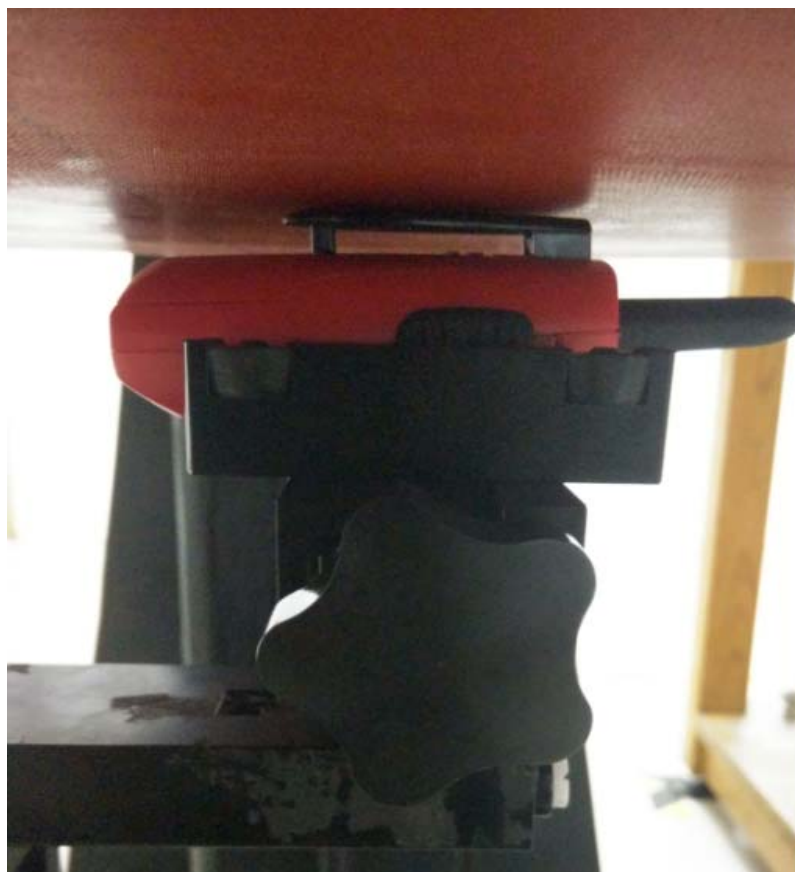
Body-worn Configuration with A1, B1, BC1 (The Belt Clip Distance was 0mm)
