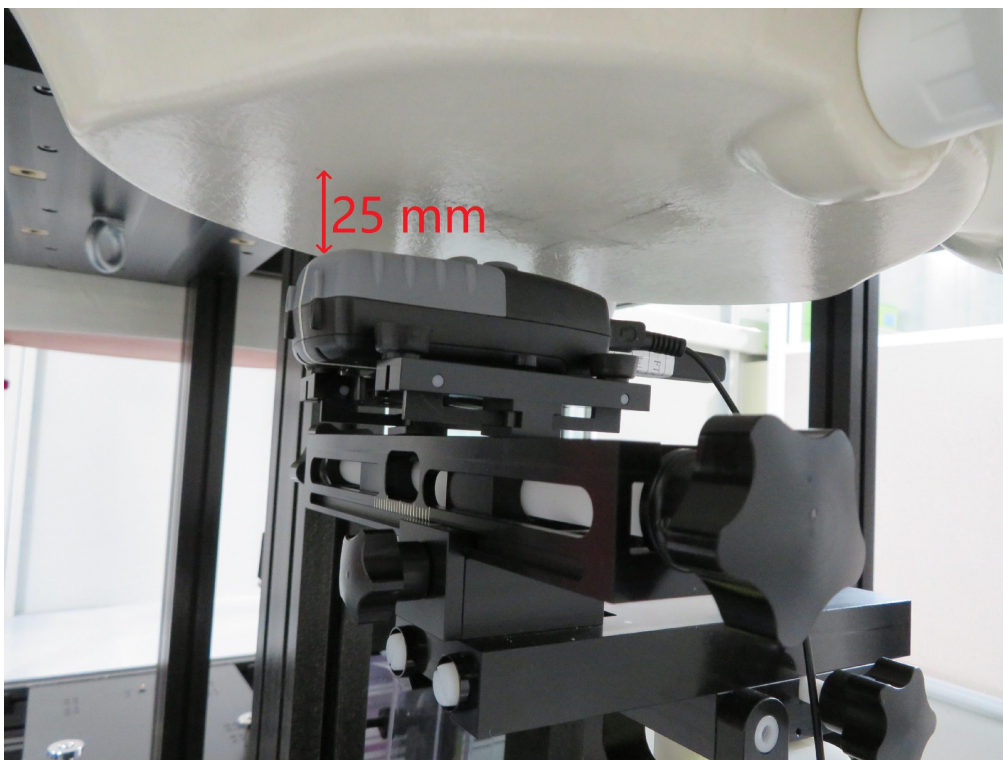
Description: Head Front of Face with earphone with 25mm gap
