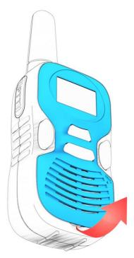
Disassemble the trim from here upwards
