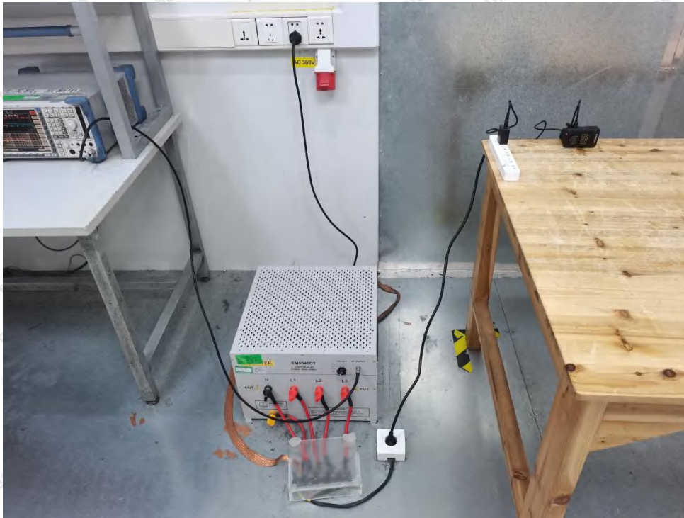
Photo of Conducted Emission Measurement
