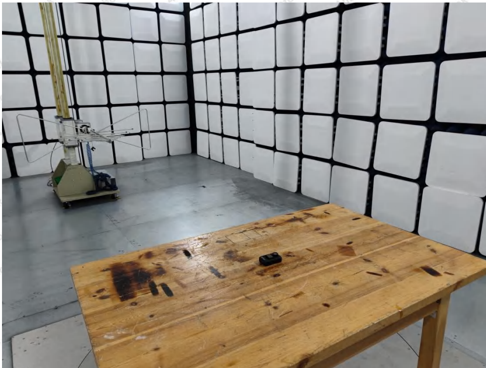
Photo of Radiation Emission Test
