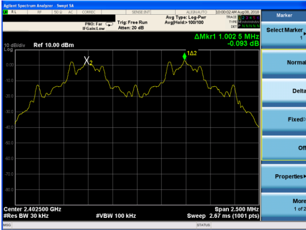
(1Mbps) Channel Separation plot on channel 39-40
