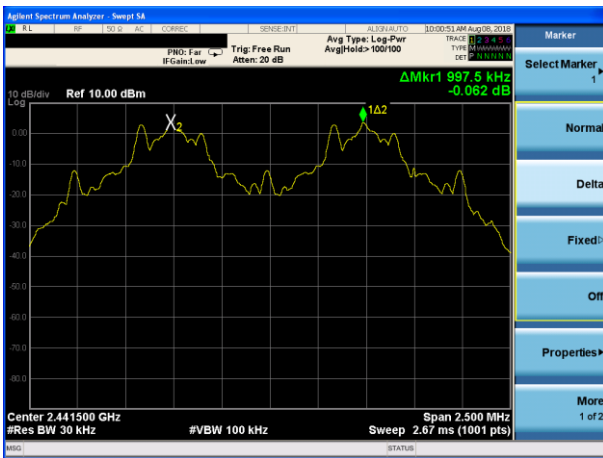
(1Mbps) Channel Separation plot on channel 77-78
