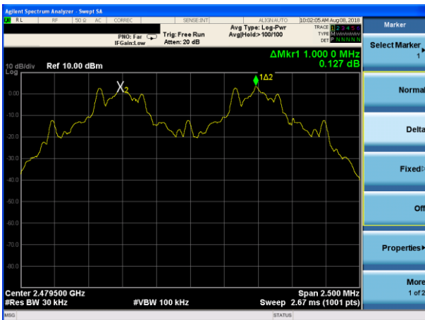
(1Mbps) Channel Separation plot on channel 77-78
