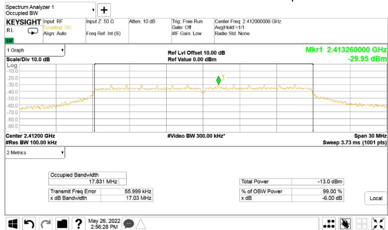
Plot 7.1.14 6 dB bandwidth test result at mid frequency
