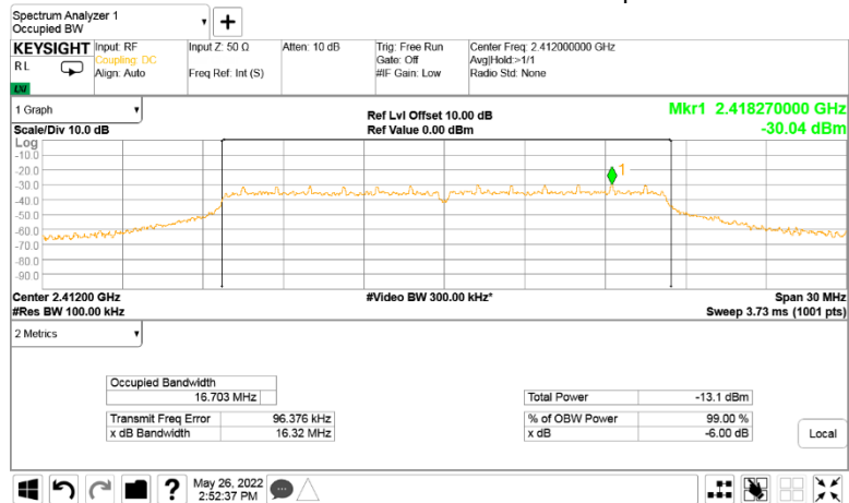
Plot 7.1.8 6 dB bandwidth test result at mid frequency
