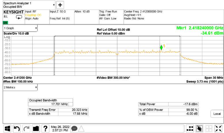
Plot 7.1.17 6 dB bandwidth test result at mid frequency
