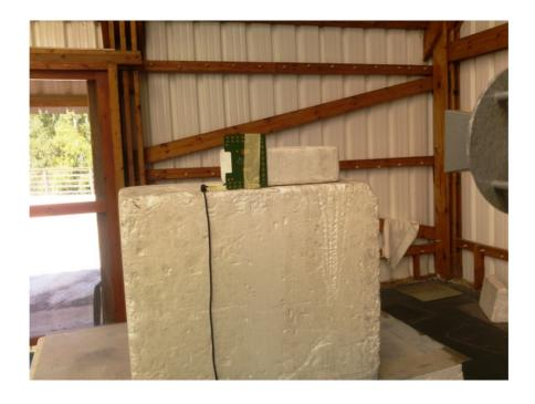
Photograph No.6 Spurious emissions measurement setup at the OATS in 18 -40 GHz
