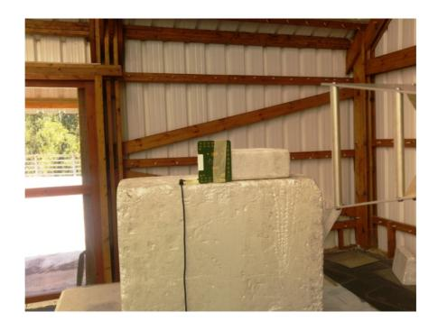
Photograph No.5 Spurious emissions measurement setup at the OATS in 1-18 GHz
