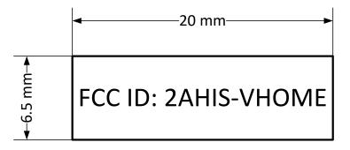
The labels will be silk-printed on the PCB, for example:
