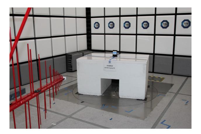
Radiated Emissions Test Setup (30MHz to 1GHz)
