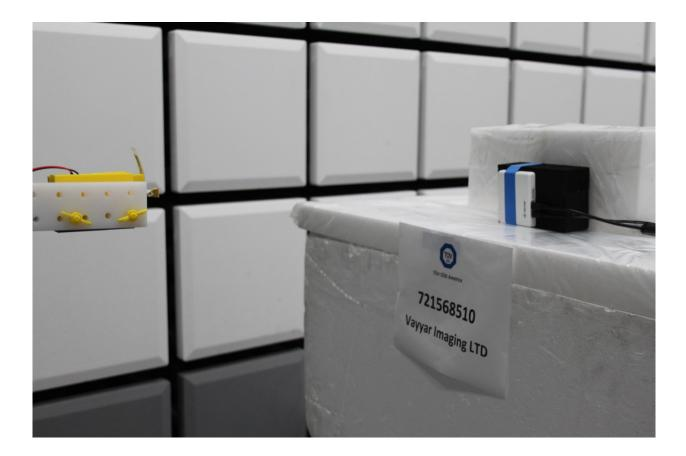
Radiated Emissions Test Setup (140GHz TO 200GHz)
