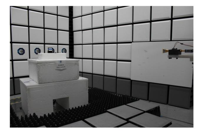
Radiated Emissions Test Setup (18GHz TO 75GHz)
