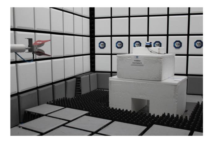
Radiated Emissions Test Setup (1GHz to 18GHz)
