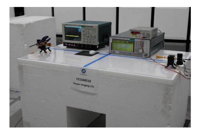
Power Measurement/Substitution Test Setup
