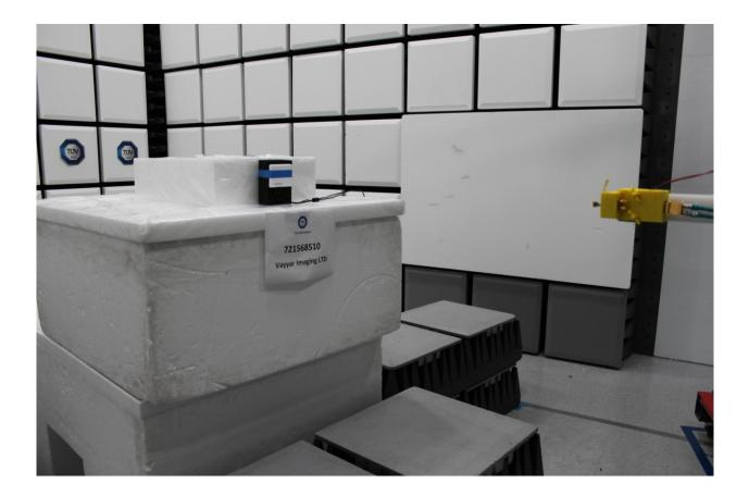
Radiated Emissions Test Setup (75GHz to 140GHz)
