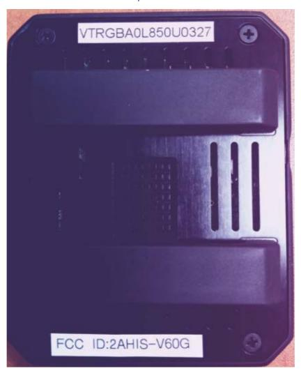
Label with **FCC ID:2AHIS-V60G** is located here. The statement according to FCC part 15 §15.19(a)(3) is placed in User Manual, page 16 (Application exhibit User\_manual\_32363).
