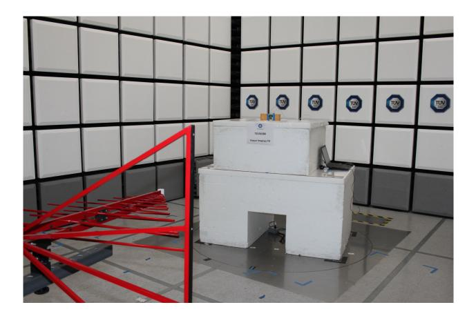
Radiated Emissions Test Setup (30MHz to 1GHz)
