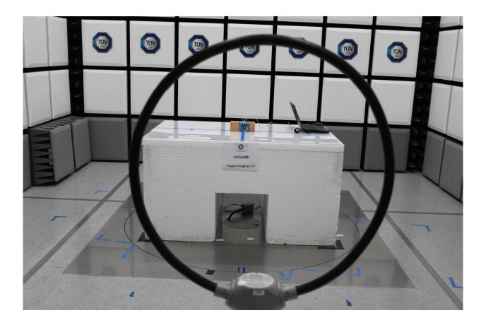
Radiated Emissions Test Setup (below 30MHz)
