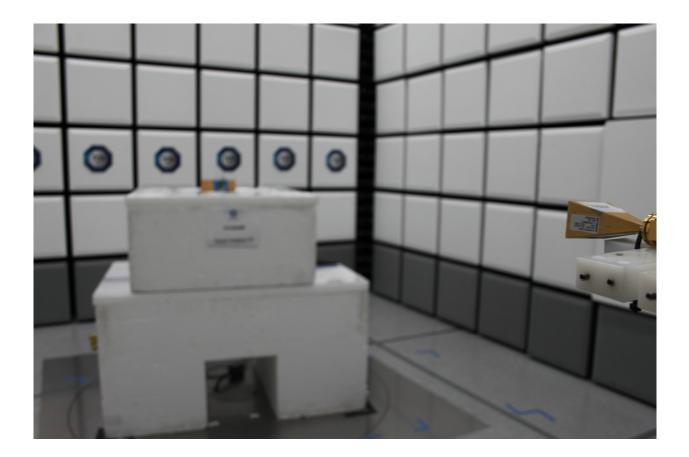
Radiated Emissions Test Setup (Above 1GHz @ 3 meters)
