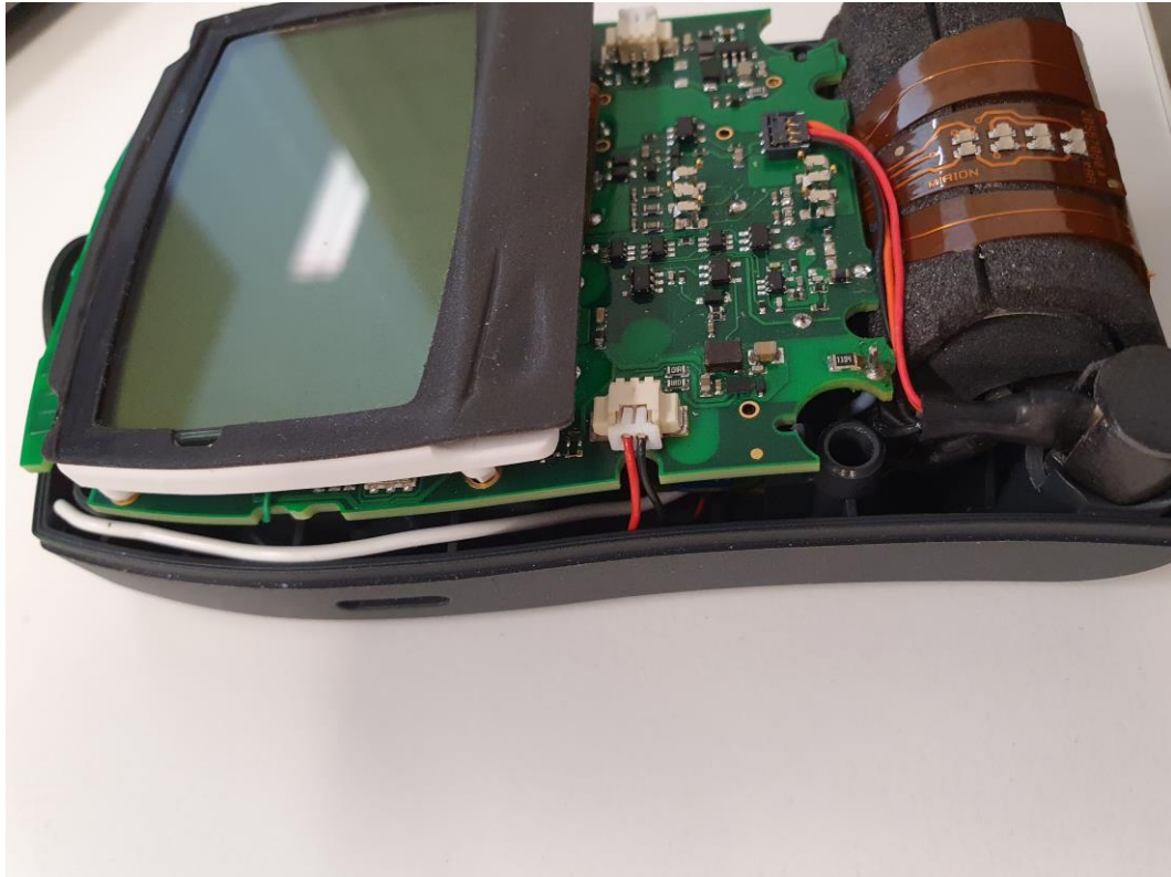
Figure 10. The positioning of the RF-module antenna within the RDS-32 casing.
