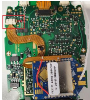
Figure 8 The positioning of the RF-module on the KRO-board.
