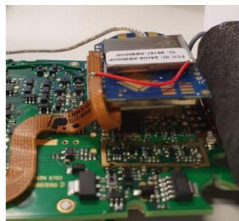
Figure 9 The positioning of the RF-module on the KRO-board
