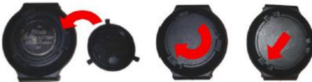
Figure 3-2: MBD-1 Battery Cover Installation
