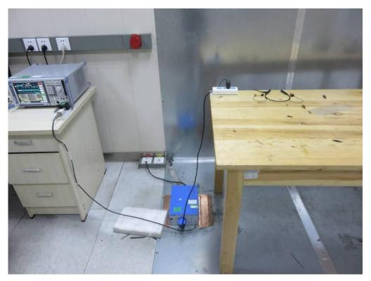
FCC RADIATED EMISSION TEST SETUP
