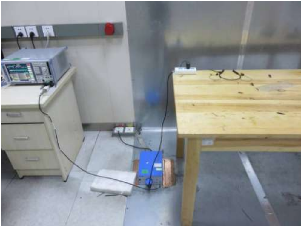
FCC RADIATED EMISSION TEST SETUP
