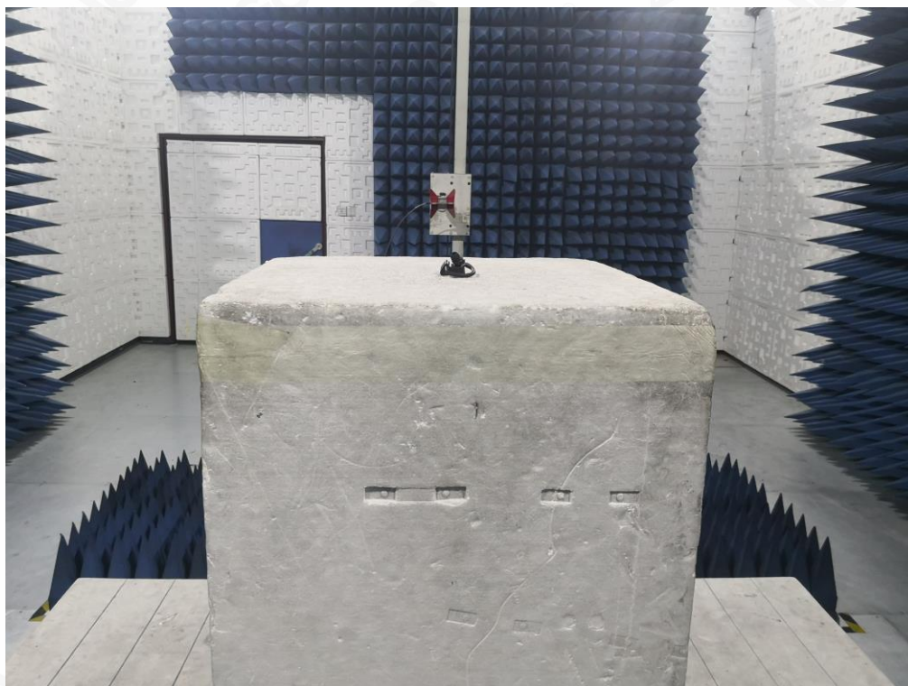
RADIATED EMISSION TEST SETUP ABOVE 1GHZ
