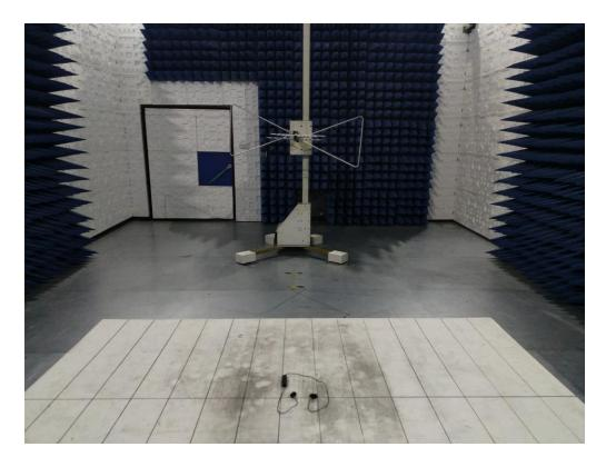
RADIATED EMISSION TEST SETUP ABOVE 1GHZ
