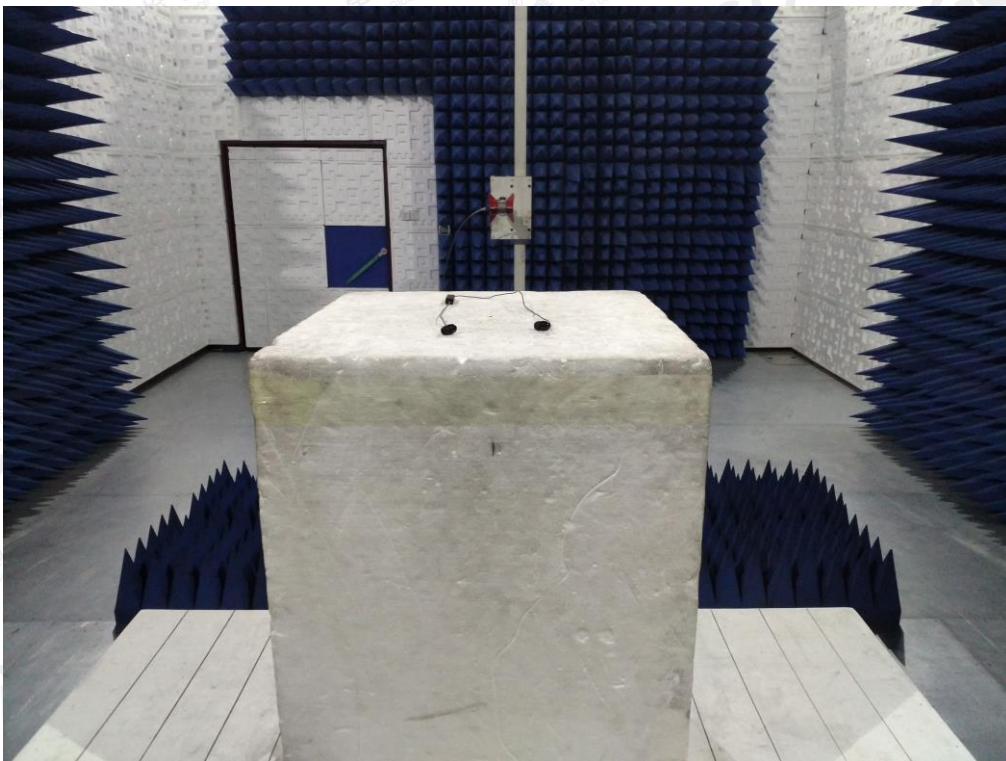
RADIATED EMISSION TEST SETUP ABOVE 1GHZ
