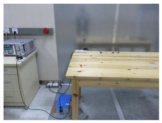
FCC RADIATED EMISSION TEST SETUP
