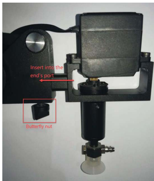
Figure 5.8 Install a suction cup kit
