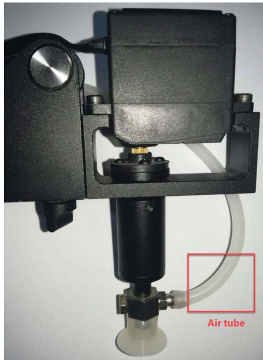
Figure 5.9 Install an air tube
