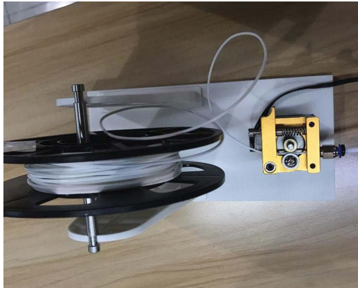
Figure 5.123 Place filament and extruder to the Filament holder
