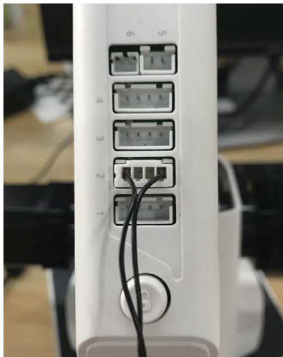
Figure 5.169 Insert the cable of the auto-levelling
