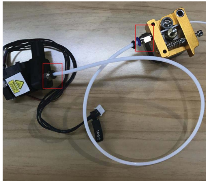
Figure 5.119 Connect extruder and hot end
