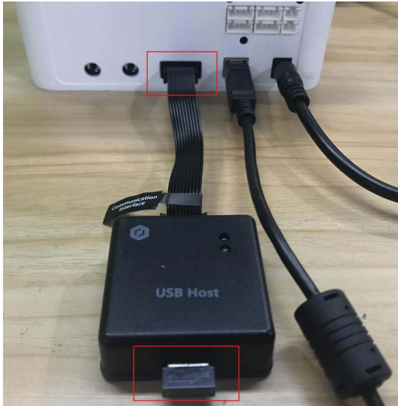
Figure 5.184 Connect with USB Host module
