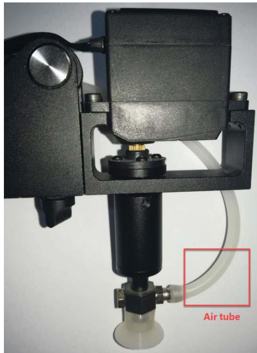
Figure 5.9 Install an air tube
