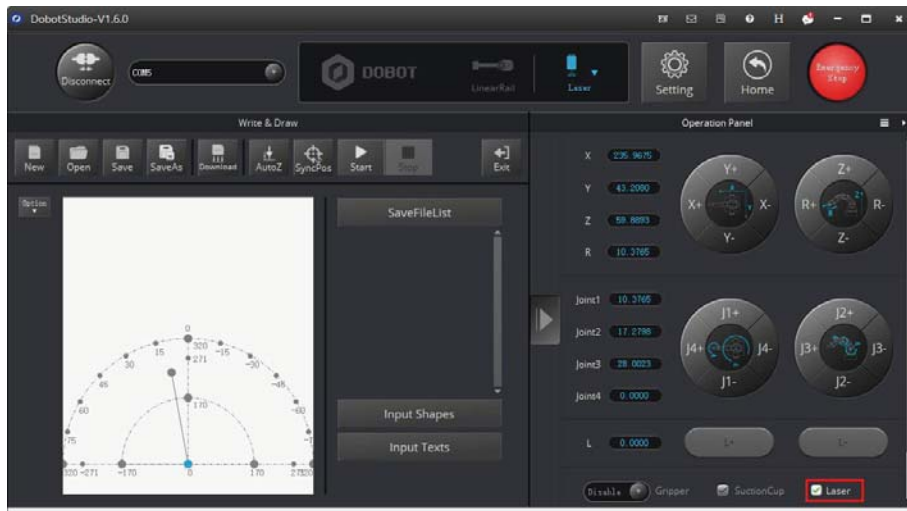
Figure 5.78 Turn on the laser
