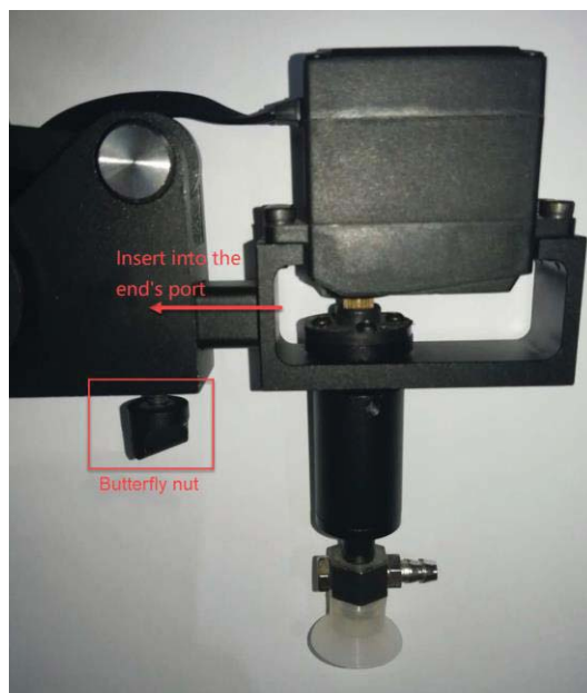
Figure 5.8 Install a suction cup kit
