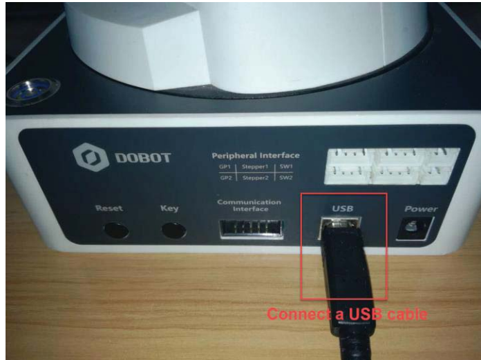
Figure 2.2 Connect the Dobot Magician to your computer
