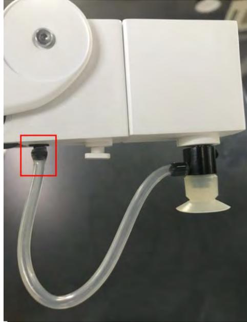
Figure 5.10 Install an air tube
