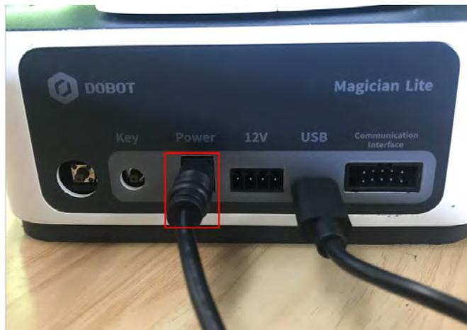
Figure 2.3 Connect Magician Lite to the electrical outlet
