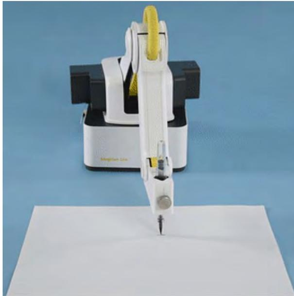
Figure 5.51 Adjust the position of the pen nib
