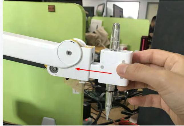
Figure 5.34 Install a writing and drawing kit
