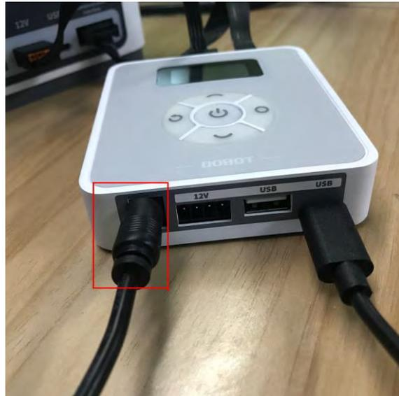
Figure 2.6 Connect power adaptor
