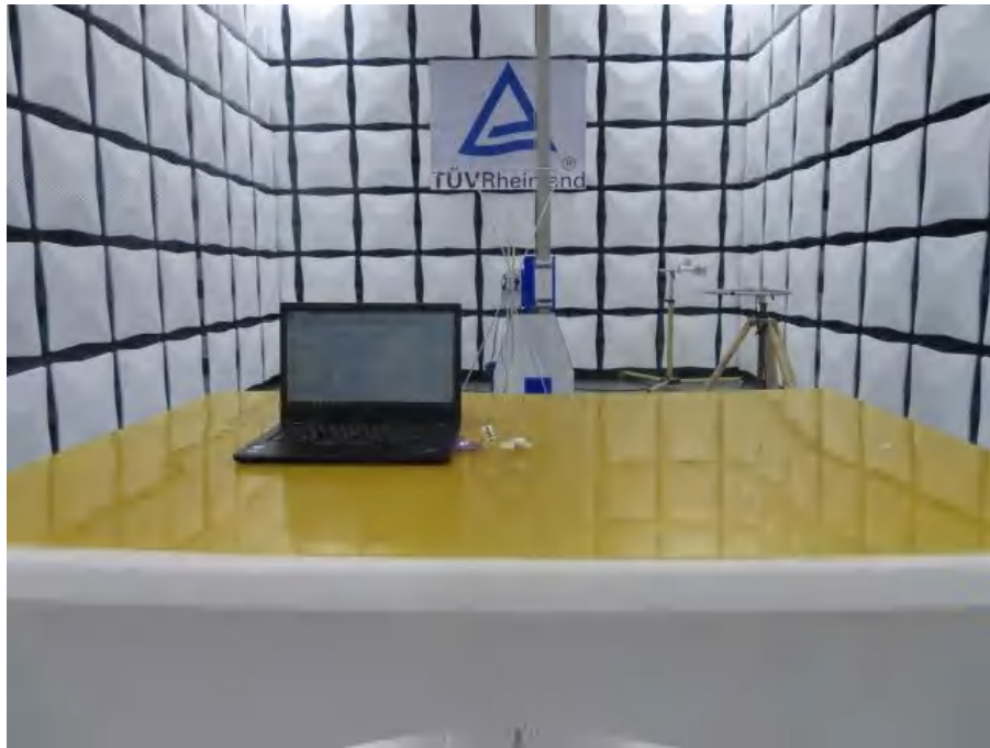
Photograph 1: Set-up for Radiated Spurious Emission, 30MHz ~ 1GHz
