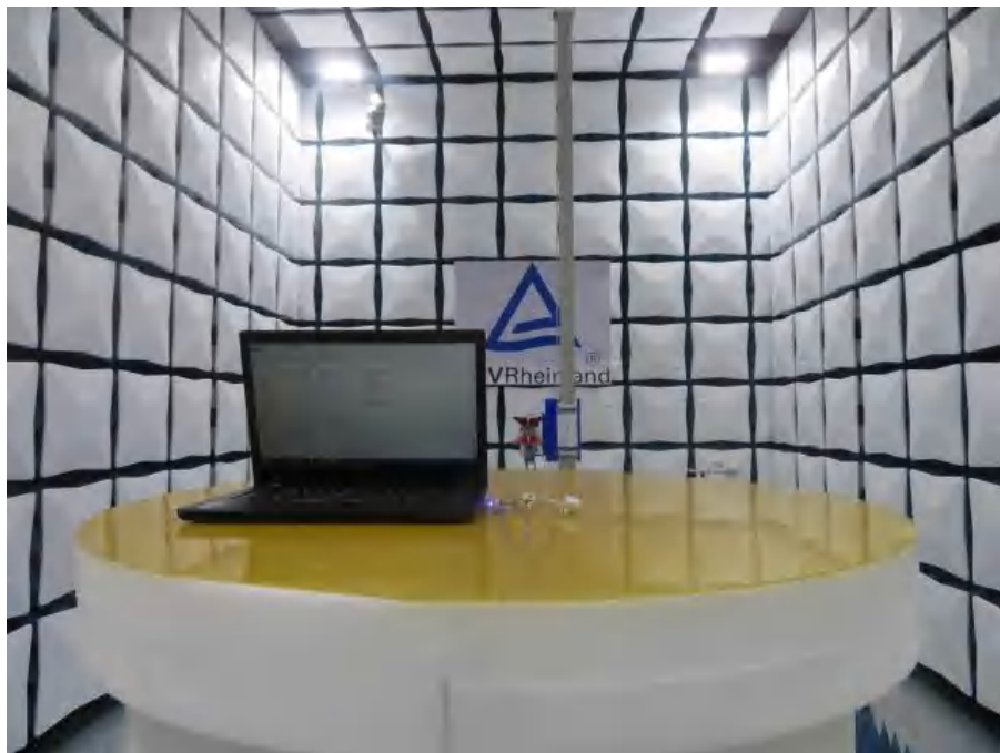
Photograph 2: Set-up for Radiated Spurious Emission, Above 1GHz
