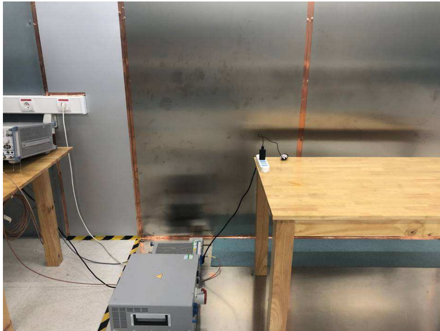
Photograph 3: Set-up for Conducted Emission on AC Mains
