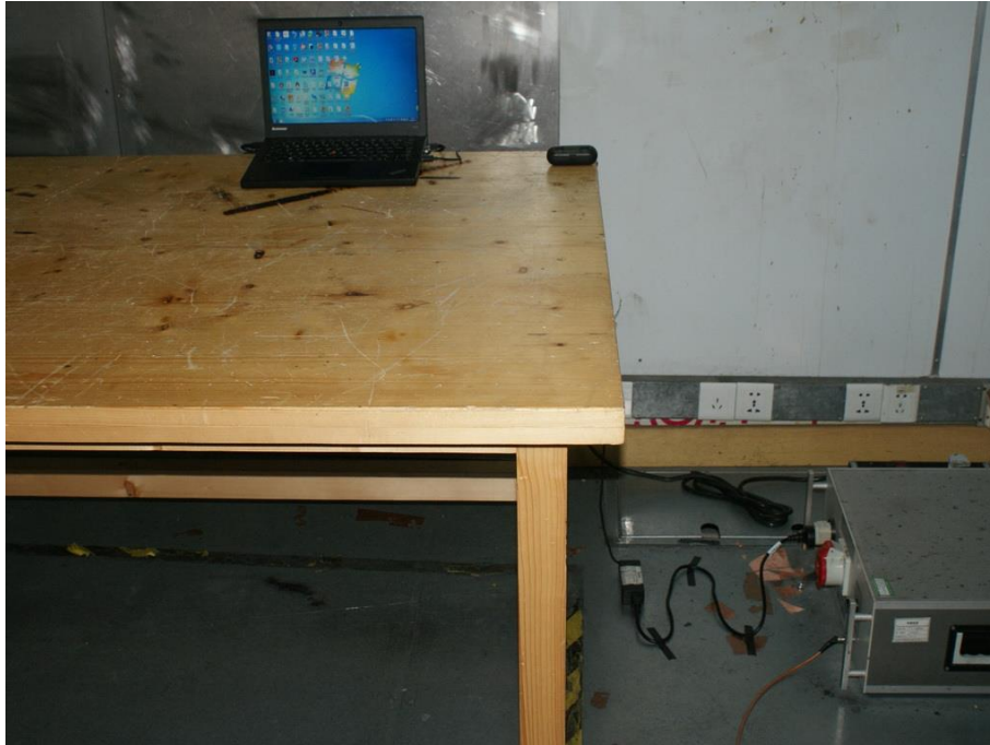
Photograph 1: Set-up for Conducted Emission on AC Mains
