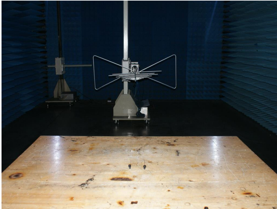
Photograph 5: Set-up for Radiated Spurious Emission, 30MHz - 1GHz
