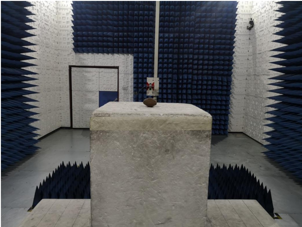
RADIATED EMISSION TEST SETUP ABOVE 1GHZ
