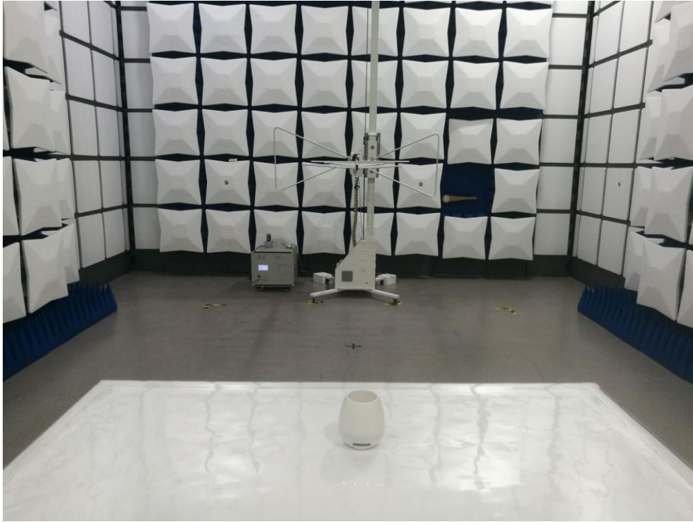
FCC RADIATED EMISSION TEST SETUP
