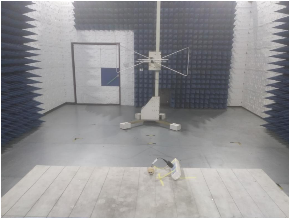
RADIATED EMISSION TEST SETUP ABOVE 1GHZ
