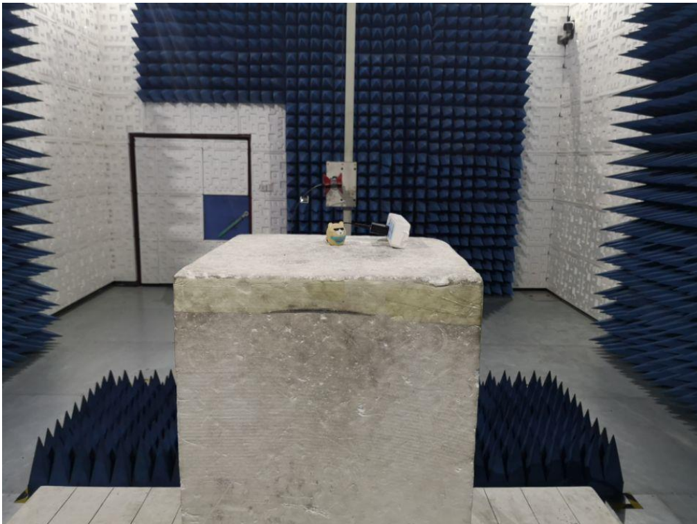
RADIATED EMISSION TEST SETUP ABOVE 1GHZ
