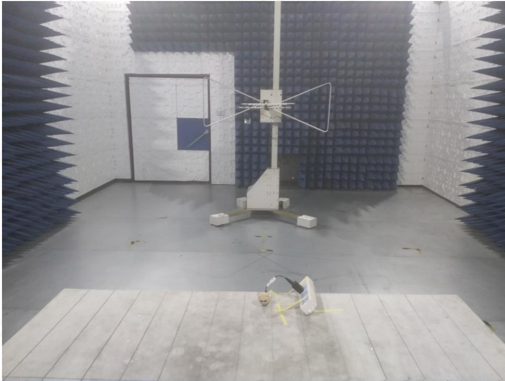
RADIATED EMISSION TEST SETUP ABOVE 1GHZ
