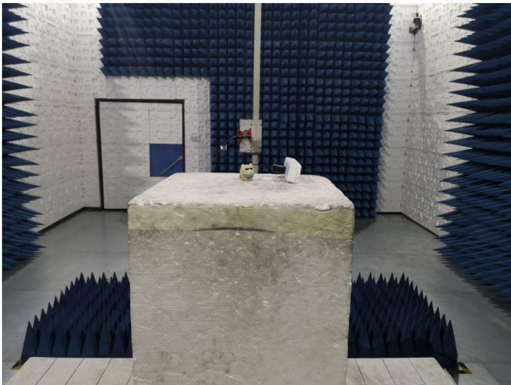
RADIATED EMISSION TEST SETUP ABOVE 1GHZ
