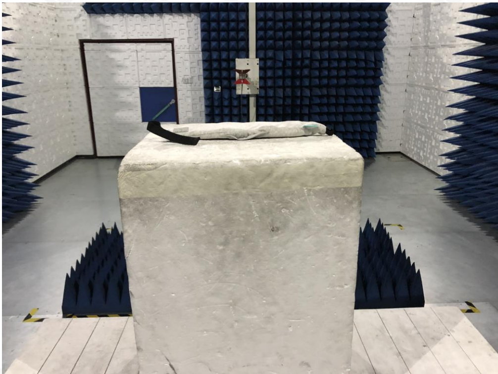
RADIATED EMISSION TEST SETUP ABOVE 1GHZ
