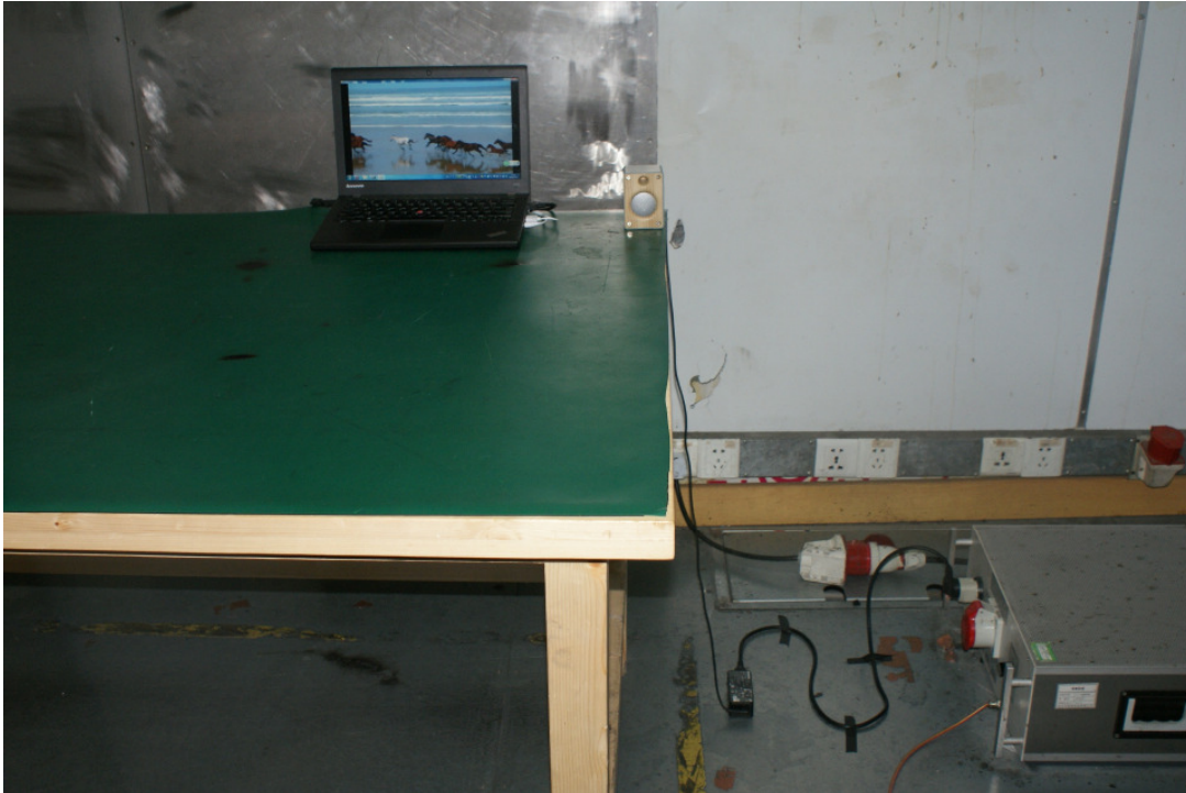
Photograph 6: Set-up for Radiated Emissions, below 1GHz
