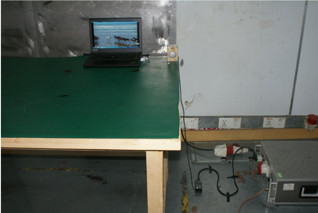
Photograph 6: Set-up for Radiated Emissions, below 1GHz
