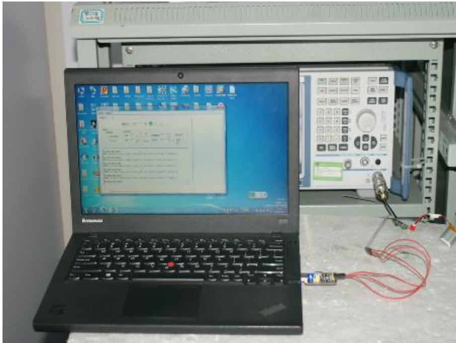
Photograph 2: Set-up for Radiated Spurious Emission (9kHz ~ 30MHz)
