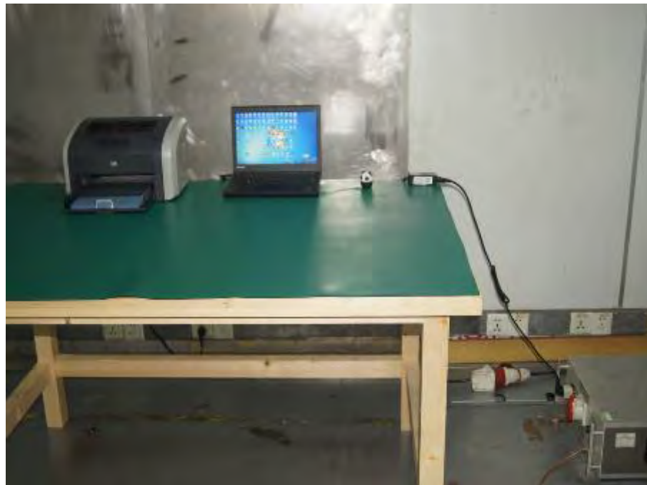
Photograph 6: Set-up for Conducted Emission
