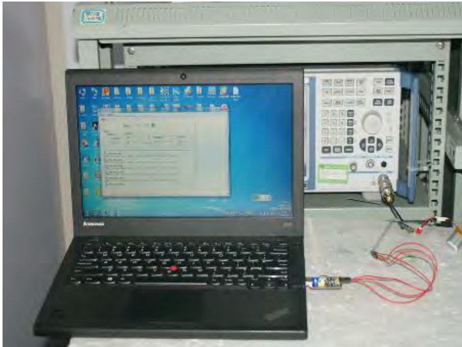
Photograph 2: Set-up for Radiated Spurious Emission (9kHz ~ 30MHz)
