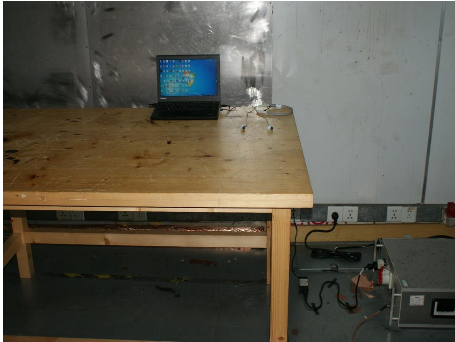
Photograph 1: Set-up for Conducted Emission on AC Mains
