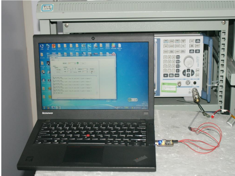
Photograph 2: Set-up for Radiated Spurious Emission (9kHz ~ 30MHz)
