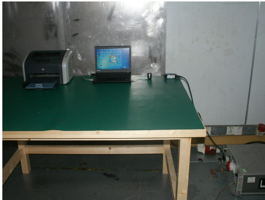
Photograph 6: Set-up for Conducted Emission
