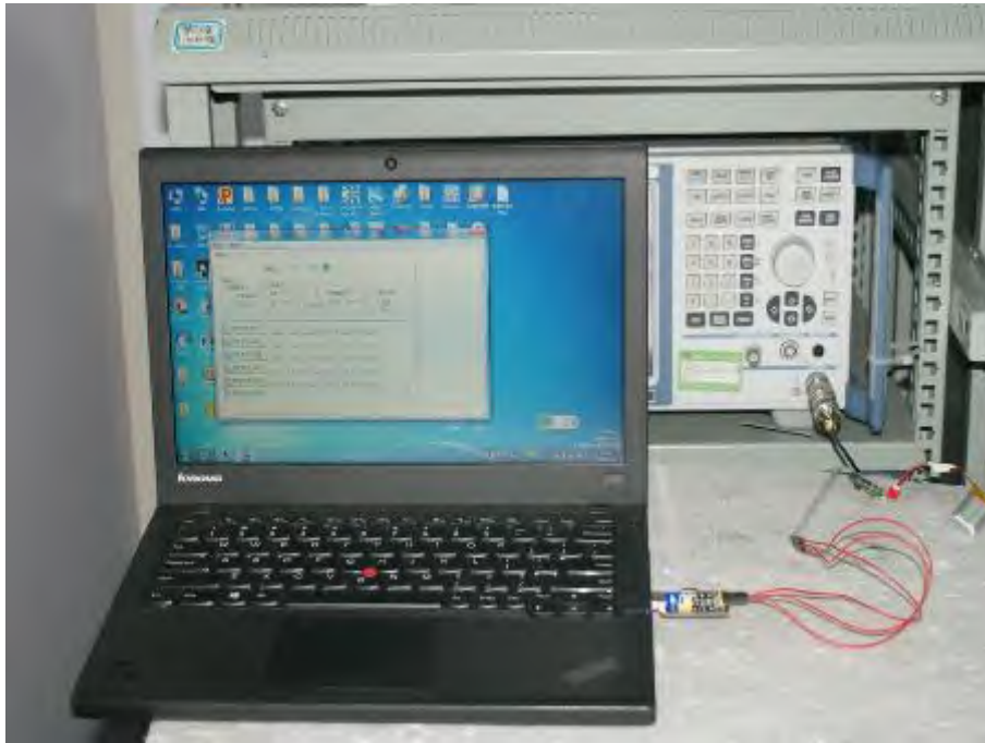
Photograph 2: Set-up for Radiated Spurious Emission (9kHz ~ 30MHz)
