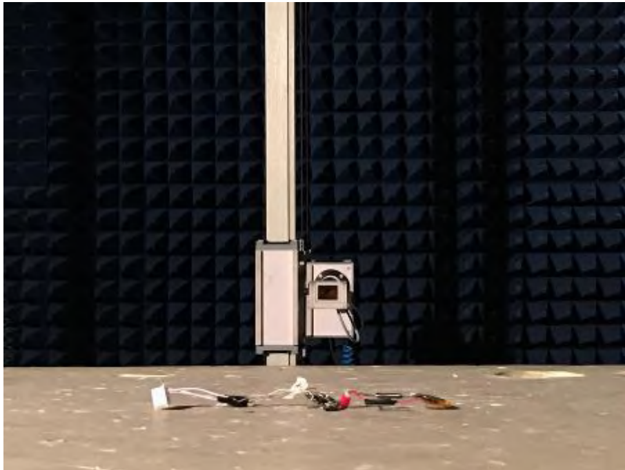
Photograph 6: Set-up for Conducted Emission
