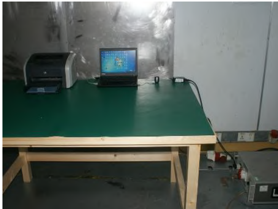
Photograph 6: Set-up for Conducted Emission
