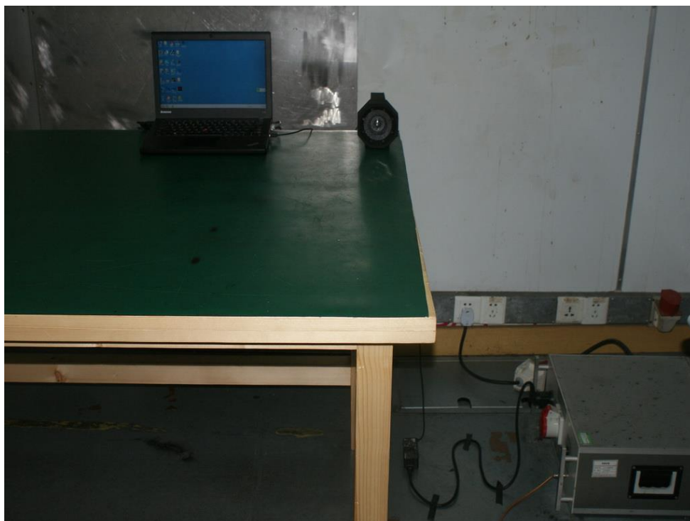
Photograph 6: Set-up for Conducted Emissions
