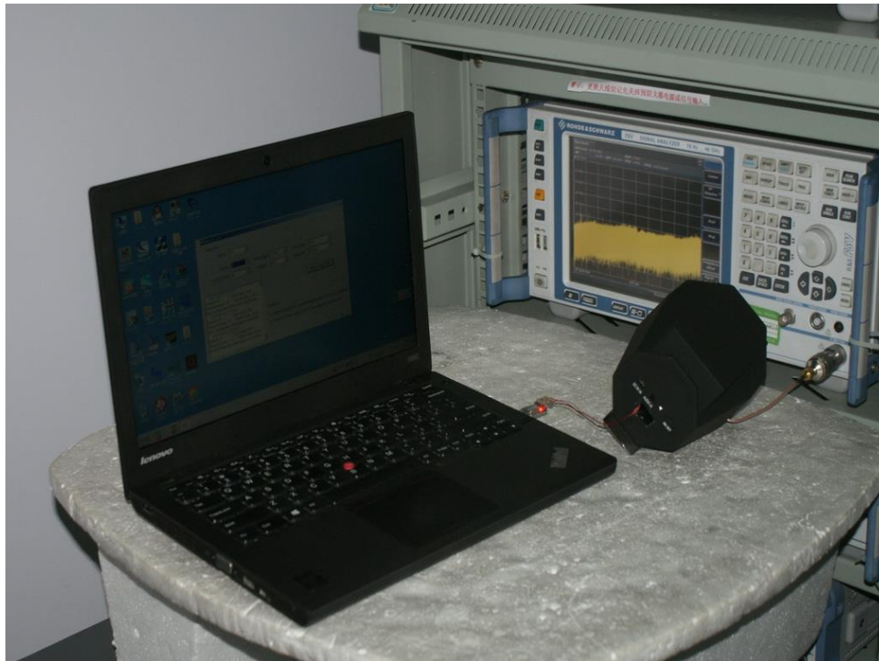
Photograph 2: Set-up for Spurious Emissions (9kHz-30MHz)
