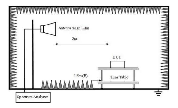
Above 1GHz Test Setup
